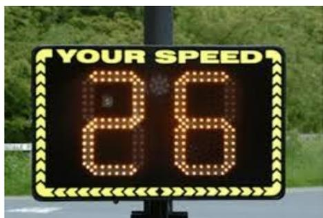
One benefit of the upgraded SIDs is that they will be mounted on removable and rotatable posts, so the two SIDs can be routinely moved between the seven locations. The devices will also enable us to collect and monitor traffic flow and speeds through downloadable data. We will use this to inform OCC of persistent issues that can then be used as preliminary evidence for future traffic calming discussions.
